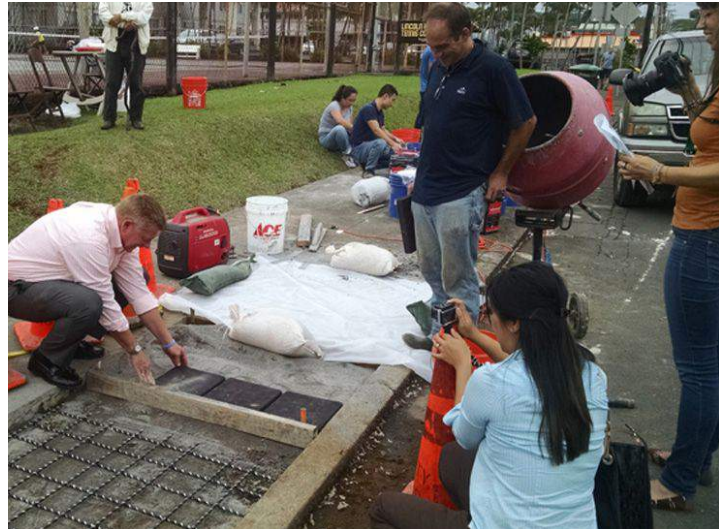
PISCES Executive Director Rob Kelso is seen here laying out the lunar concrete at our test site in downtown Hilo, Hawai'i.
